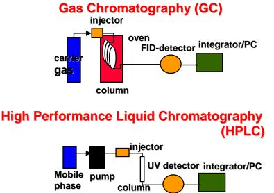
The FID detector is a Flame Ionisation Detector which analyses for all organic compounds. The HPLC uses a Ultra-Violet Detector which analyses for those organic compounds which contains a chromaphoric group.
