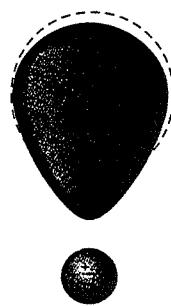
Figure 14.3 The effect of \text{Li}^+ charge density on a nearby electron cloud. The ability of the \text{Li}^+ ion to deform nearby electron clouds gives rise to many anomalous properties for a Group 1A(1) element. In this case, \text{Li}^+ polarizes an \text{I}^- ion, which gives some covalent character to lithium iodide, \text{LiI} .
